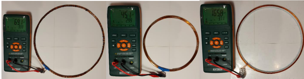
Fig. 2. Checking self-inductors of planar loop coils
