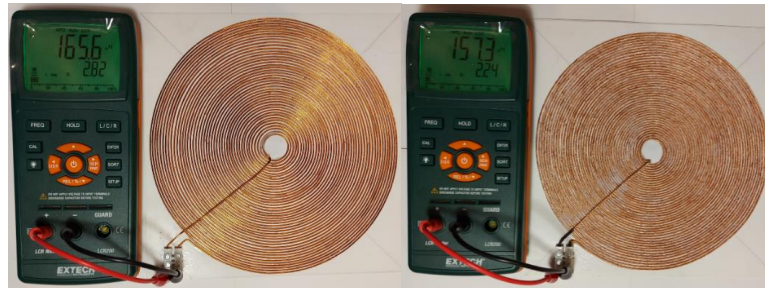
Fig. 3. Checking self-inductance planar spiral coil
